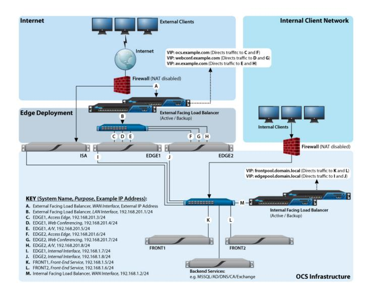
As shown in <u>Figure 1</u>, the firewall should not NAT inbound traffic addressed to the Edge deployment.
