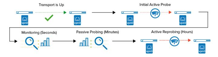
For UDP transports, the firewall can determine the actual bandwidth available for a VPN transport through monitoring, active probing, and passive probing. Dynamic bandwidth and Round Trip Time detection is available for IPv4 connections only . To have a valid starting point, the initial bandwidth is set in the VPN transport configuration. The goal for the link-quality probing is to find the settings that
