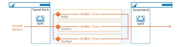
Adaptive Session Balancing uses link-quality metrics collected by Dynamic Bandwidth and Round Trip Time Detection for both the initial balancing and to rebalance sessions with a lifetime over 5 seconds.
