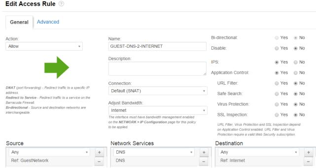
To allow connections from the guest network to the Internet, the X-Series Firewall must perform source-based NAT. The source IP address of outgoing packets is changed from that of the client residing in the network to the WAN IP address of the X-Series Firewall, so the connection is established between the WAN IP address and the destination IP address. The destination address of reply packets belonging to this session is rewritten with the client's IP address.
