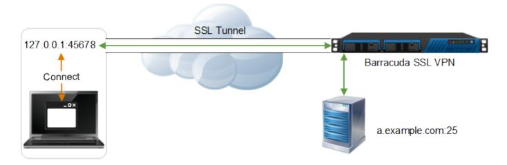
SSL tunnels can be configured to only allow local connections or to allow connections directly to the remote network. It is also possible to define the source IP address of the SSL tunnel, so that clients in the same remote network can share a SSL tunnel. The tunnel is terminated when the session is closed or timed out.
