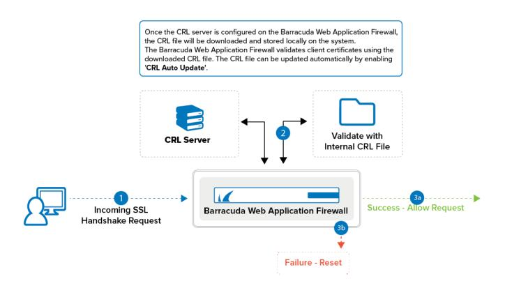
The Barracuda Web Application Firewall uses the default gateway or a static route to access the server hosting the CRL.
