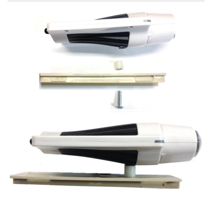
**Step 6: Secure Camera Mount and Control PCB**
