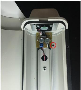
3. Using the supplied lock washer and nut, install the RP-SMA extension cable into this hole.
