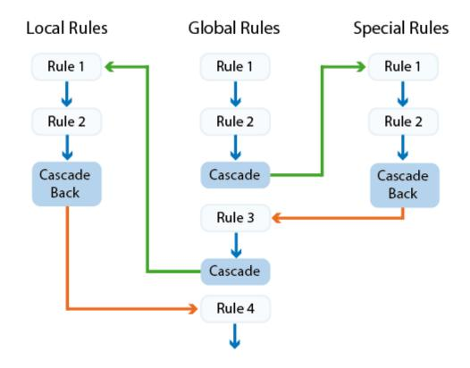
The workflow of rules in the **Global Rules** section is intercepted through cascading to either **Special**-or **Local Rules** section. As a final step, from there the workflow is returned to the **Global Rules** section with a **Cascade Back** rule.
