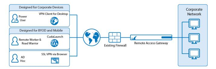
You can now deploy your X-Series Firewall as a remote access gateway behind your border firewall. This allows you to leverage the remote connectivity options offered by the SSL VPN and client-to-site VPN services on the X-Series Firewall to offer easy remote connectivity for all your users. The remote access gateway wizard can be launched separately or during the deployment.
