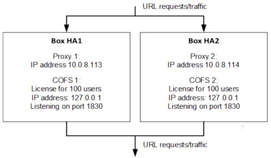
If Box HA-2 is down (for example, because of a hardware failure), Box HA-1 takes over the proxy server and URL filter server that were hosted by it.
