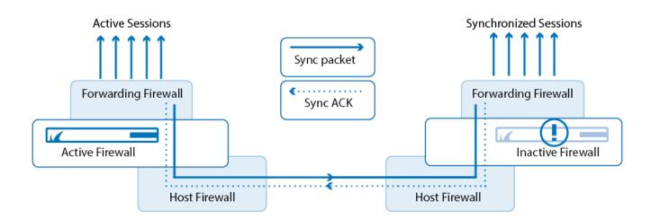
The synchronizing procedure takes place immediately (if possible). If synchronization packets are lost, up to 70 sessions per second are synchronized.
