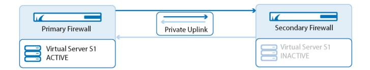
When configuring HA without a private uplink, the switch both firewalls are connected to represents a single point of failure. If traffic is not forwarded by the switch, the HA sync breaks because the primary and secondary unit cannot establish a connection. To always have a reliable connection, you can configure a private uplink.
