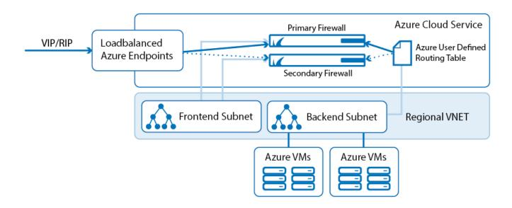
To be able to run a high availability cluster for firewalls running in Microsoft Azure, a special setup is required to integrate in to the Azure networking environment.
