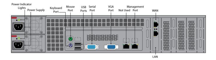
The following table describes the Barracuda Web Security Gateway 1010 rear panel ports and connectors. **NOTE:** Functionality of the WAN, LAN and AUX port lights vary by vendor.
