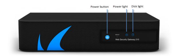
The following table describes the Barracuda Web Security Gateway 210 front panel power and disk activity indicator lights.
