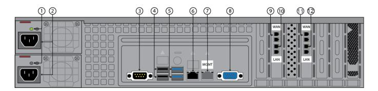
The following table describes the Barracuda Web Security Gateway 1011 rear panel ports and connectors. **NOTE:** Functionality of the WAN, LAN and AUX port lights vary by vendor.
