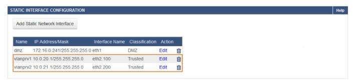
Go to **NETWORK** > **Routing**. If no errors occurred during the configuration, you can see the two VLAN interfaces in both the **Network Routes** and the **Network Interfaces** tables.
