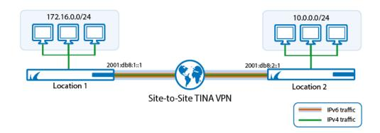
Site-to-Site VPNs establish secure connections between two locations over a public network such as the Internet. The proprietary TINA protocol offers intelligent traffic management capabilities using Traffic Intelligence, WAN optimization, and on-the-fly traffic shaping. For connectivity with third-party VPN gateways, it is also possible to create Site-to-Site VPN connections using IPsec.
