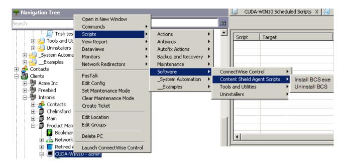
ConnectWise connects to the remote agent and passes on the execution command to the client machine, where the script is executed. You can view information about the client and follow script activity by double-clicking the client machine in the Navigation Tree. There is a script section where you can find information about scripts that have been scheduled, queued, or already executed.
