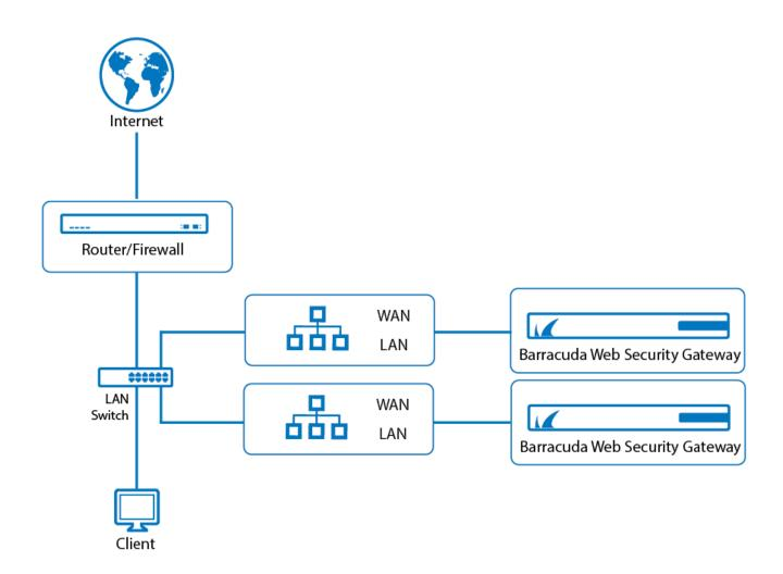
Figure 2 below shows deployment with a WCCP router for filtering both HTTP and HTTPS traffic. In this deployment, the Barracuda Web Security Gateway uses a physically separate gateway to the internet relative to the WCCP router. This configuration is appropriate if your switch does not support VLANs and you want to filter both HTTP and HTTPS traffic with your WCCP router. See the **BASIC** > **IP Configuration** page to select and configure WCCP deployment.
