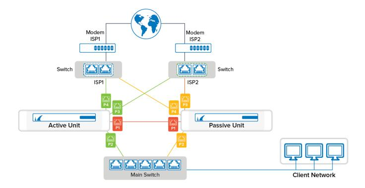
To configure High Availability, simply select two appliances during the deployment while creating the site configuration or when adding a new site. Both appliances must be the same model and have the same firmware version.
