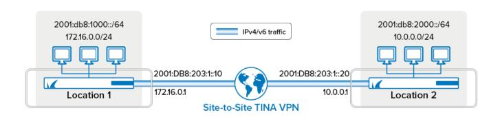
TINA is a Barracuda Networks proprietary VPN protocol designed to extend the feature set and to remove the limitations of the IPsec protocol. TINA is designed to provide superior VPN connectivity and availability. Site-to-Site TINA tunnels can be established only between CloudGen Firewalls. Advanced VPN features, such as SD-WAN or WAN Optimization, are available only for TINA VPN tunnels. TINA tunnels support both IPv4 and IPv6 VPN traffic.
