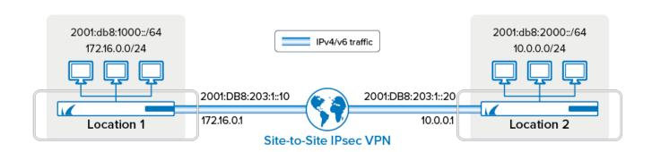
IPsec has established itself as the standard for VPN tunnels and is widely supported by almost all VPN device manufacturers. The Barracuda CloudGen Firewall supports both IKEv1 and IKEv2 IPsec Site-to-Site VPN tunnels to third-party VPN devices. IPv6 is supported only for IKEv2 IPsec tunnels.
