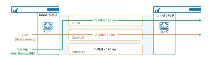
Performance-Based Transport Selection selects the optimal transport based on the policy selected in the SD-WAN settings of the custom connection object. Only UDP transports with Dynamic Bandwidth and Round Trip Time Detection enabled are included in the Performance-Based Transport Selection policy. The transport selections are made from the point of view of the SD-WAN primary. The following policies are available:
