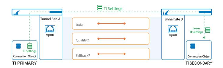
Multi-transport VPN tunnels can be configured either manually for each TINA site-to-site VPN tunnel, or via the GTI Editor if both firewalls are managed by the same Firewall Control Center. The SD-WAN settings of the custom connection object used in the matching access rule determines which transport is used. In addition to transport balancing, failover, and advanced bandwidth management, features can be enabled to fully utilize all available WAN connections.
