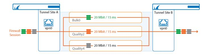
Packet-based balancing requires transports with the same Round Trip Time and bandwidth, for example multiple identical WAN links from the same ISP. The VPN traffic is balanced with a round robin balancing policy on a per-packet basis over multiple VPN transports. Packet-based balancing is enabled in the TINA VPN tunnel configuration.
