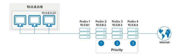
A **Cache Peer Access** filter must be set for ProxySrv2 and a **Domain Restrictions** filter must be set for ProxySrv3. ProxySrv4 is set up without any filters, which means that all requests that do not match the configured filters will be directed to it.
