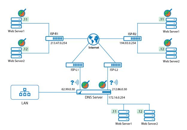
The solution is to monitor the remote web servers in the two regions R1/R2 using health probes. These health probes must be configured to monitor ports 80/443 on the respective web servers. It is not necessary to use health probes for the internal web servers in the DMZ because in this example it is assumed that both web servers will be available all the time. By configuring 2 listeners, incoming
