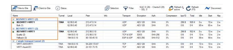
Verify the intended traffic is using the intended transport by checking the **SD-WAN ID** column in **Firewall > Live** and **Firewall > History** .
