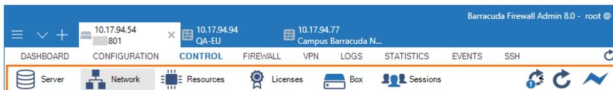
In the top-right corner, the ribbon bar provides icons to specify system refresh settings. Clicking the last icon disconnects the unit. When disconnected, this icon changes to **Connect**.
