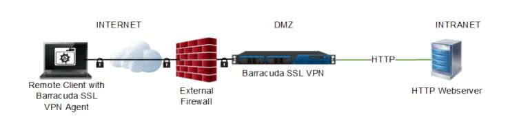
The Barracuda SSL VPN Agent is used to tunnel unencrypted connections. The traffic is intercepted and rerouted by the SSL VPN Agent installed on the client computer and then sent through a SSL encrypted tunnel to the Barracuda SSL VPN.
