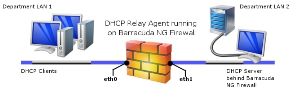
Figure 1. DHCP relay agent between two LANs.
