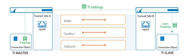
Multi-transport VPN tunnels can be configured either manually for each TINA site-to-site VPN tunnel, or via the GTI Editor if both firewalls are managed by the same NextGen Control Center. The TI settings of the custom connection object used in the matching access rule determines which transport is used. In addition to transport balancing, failover, and advanced bandwidth management, features can be enabled to fully utilize all available WAN connections.
