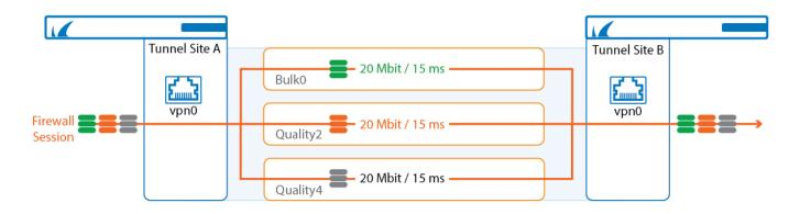
Packet-based balancing requires transports with the same latency and bandwidth, for example multiple identical WAN links from the same ISP. The VPN traffic is balanced with a round robin balancing policy on a per-packet basis over multiple VPN transports. Packet-based balancing is enabled in the TINA VPN tunnel configuration.
