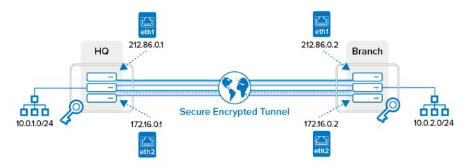
If the preferred tunnel enveloping connection fails to be established, it cannot be rebuilt automatically. The tunnel must be terminated manually. It is then immediately rebuilt with the specified algorithm. The setup depicted in the above example uses the following settings:
